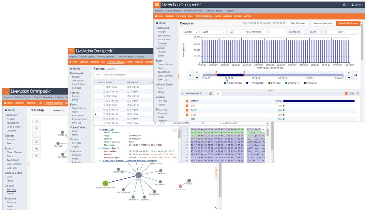
The screen below shows the *Packets* view in Omnicap which displays the list of packets and various other details about them, including the Experts, decode, and Hex view for each one.
